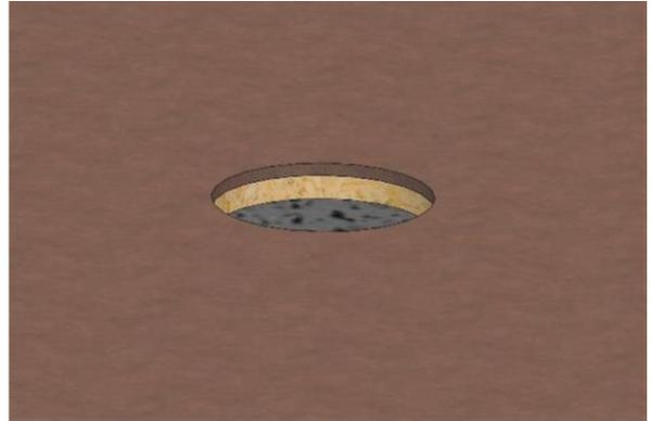
A hole of approx. Ø152 mm is drilled in the required place of the floor.
