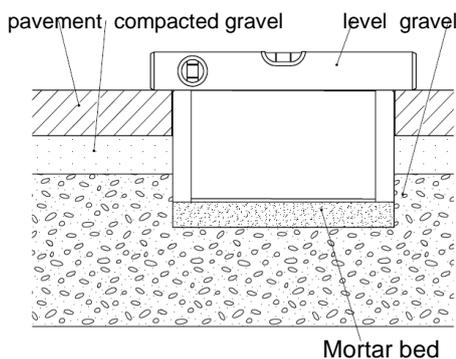
Use a spirit level to push the floor box into a mortar bed, etc. or similar material and level it with the final terrain
